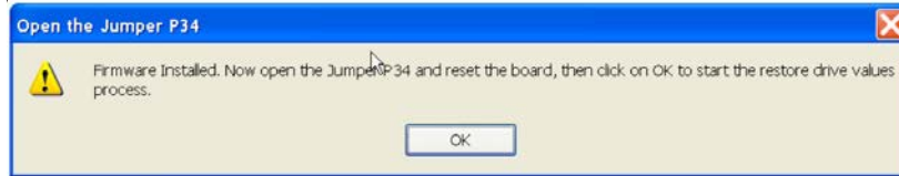
Figure F.9 – Download Firmware. Open the jumper
