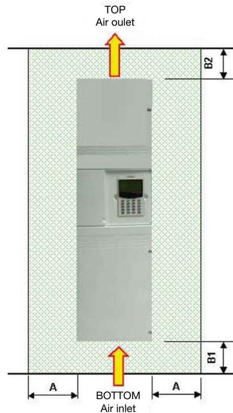
Figure 5.3.1 Free space near the drive
